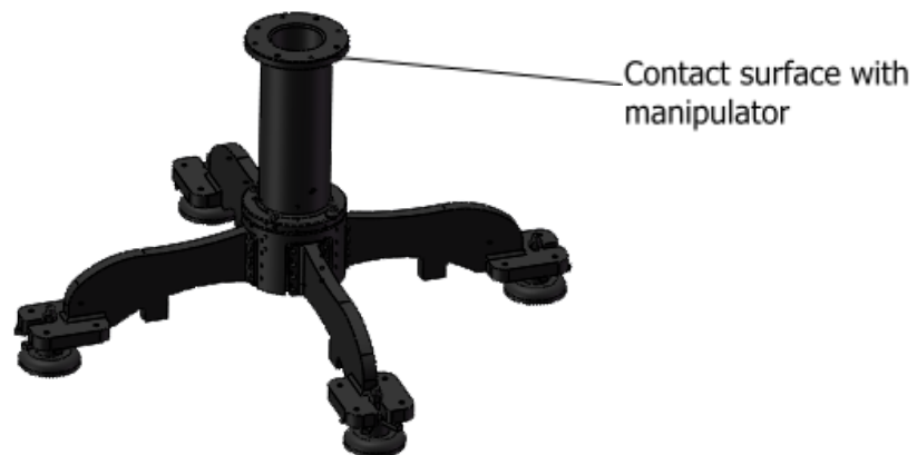
Figure 6-3 Diagram of manipulator base structure
