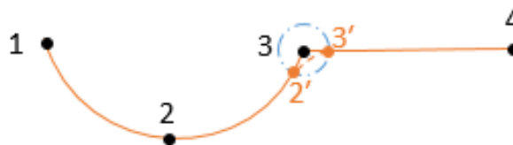
Figure 11-40 Arrival Ahead – Blend Radius, Move Arc – Move L Trajectory Example
