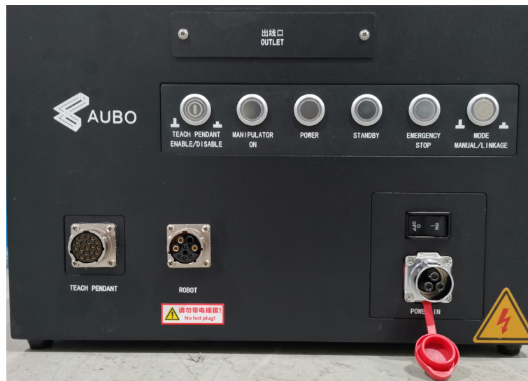
Figure 7-2 Front panel of the control box
