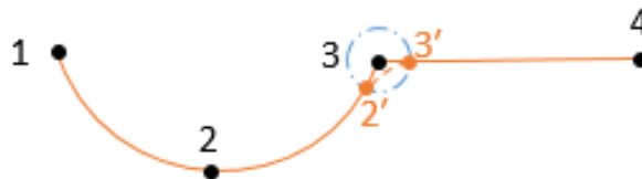
Figure 11-40 Arrival Ahead – Blend Radius, Move Arc – Move L Trajectory Example
