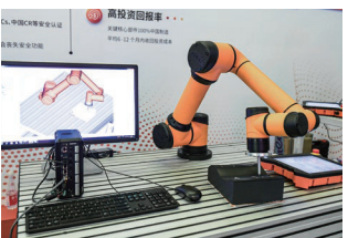
Robot with digital twin technology
