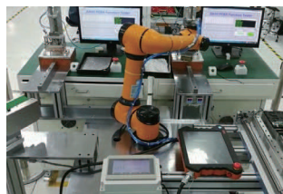
Inspection of circuit boards
