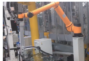
Gluing of vehicle windows
